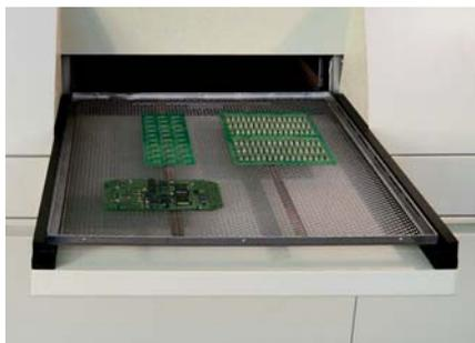
Feed-In with Work-Piece Carrier and a Variety of Assemblies
