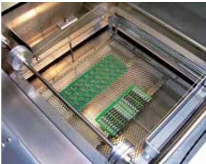
Thanks to variable temperature gradient control, a certain amount of vapour, which is adapted to the respective heat required by the modules, is automatically created. This means that the optimum tempera-
